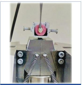
[Table/Fig-2]: Shear bond strength test.
